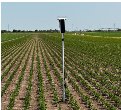
Figure 2. Installation of Arable Mark 3 in field in Nebraska
